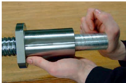
Fig. 4.6 Screw nut with wiper onto shaft
