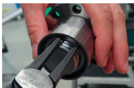
Fig. 4.9 Removing the circlip
