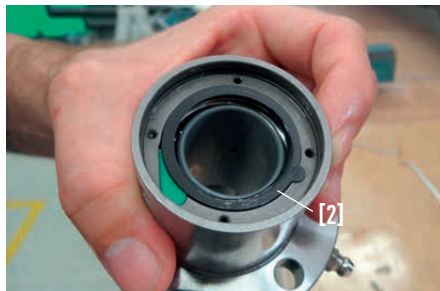
Fig. 4.12 NBR wiper [2] and support ring [1]
