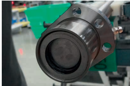
Fig. 4.10 Removing the metal ring
