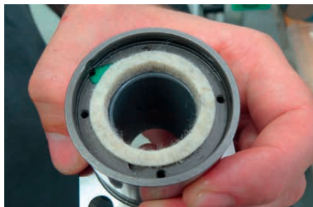
Fig. 4.13 Nut with inserted felt wiper
