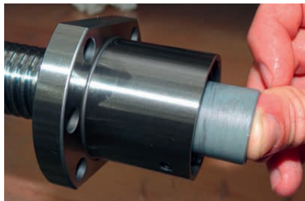
Fig. 4.11 Disassembly of the nut using an assembly tube
